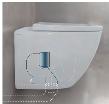
Vaso scarico universale traslato filo muro Shifted universal outlet back to wall wc
